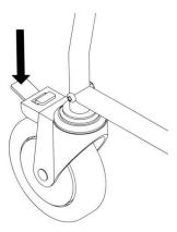
Press down on the lever located above the wheel to apply the castor parking brake (as shown in the diagram). To release the lock, press the protruding tab above thewheel.
