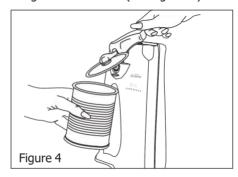
CAUTION: Be careful when removing the lid from the magnet as the cut edge is sharp. Opening dented/damaged cans: Occasionally, badly dented cans will cause the Open All™ can opener to stall. If this happens, grasp the dented can and guide it through the cutting action manually until the damaged areas are opened.
